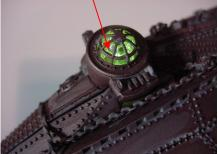
Main interior area X-4 Use 4.8 mm warm white Use 1.5 K resistor on circuit board Wire length cut to fit Close = bright / Back set = dim
